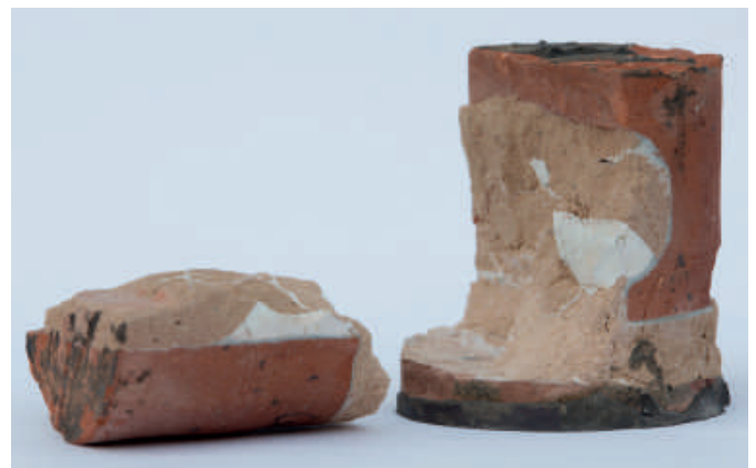
Core sample showing evidence of successful latex-cement injection (white)
